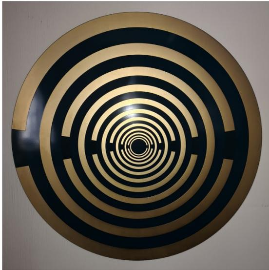
Antenne MWO 100 mm, plaqué or double face
